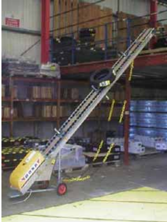
Figure 2. A conveyor used to transport tyres to and from a mezzanine floor store.
