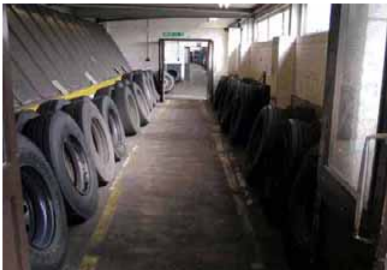
Figure 14. Good practice. Large tyres kept vertical makes collecting and rolling them easy.
